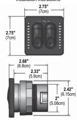
Align the centre bit of a 2 1/16" (5.24cm) hole saw with the cross hairs in the centre of the desired mounting area and drill straight down through the console, providing additional clearance for switch and electrical connection. Insert the switch into the console cutout then hand tighten the Bezel Locknut clockwise onto the back side of the key pad.
